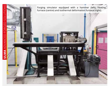
**MONDRAGON** Unibertsitatea and ULMA Advanced Forged Solutions have developed a hot forging emulator to study the recrystallization mechanisms of super-alloys and critical materials. The **objective** of this facility is to emulate, beforehand, the forging processes used at the Oñati and Lazkao plants and to optimize the final process design by reducing the current trial and error phases.
